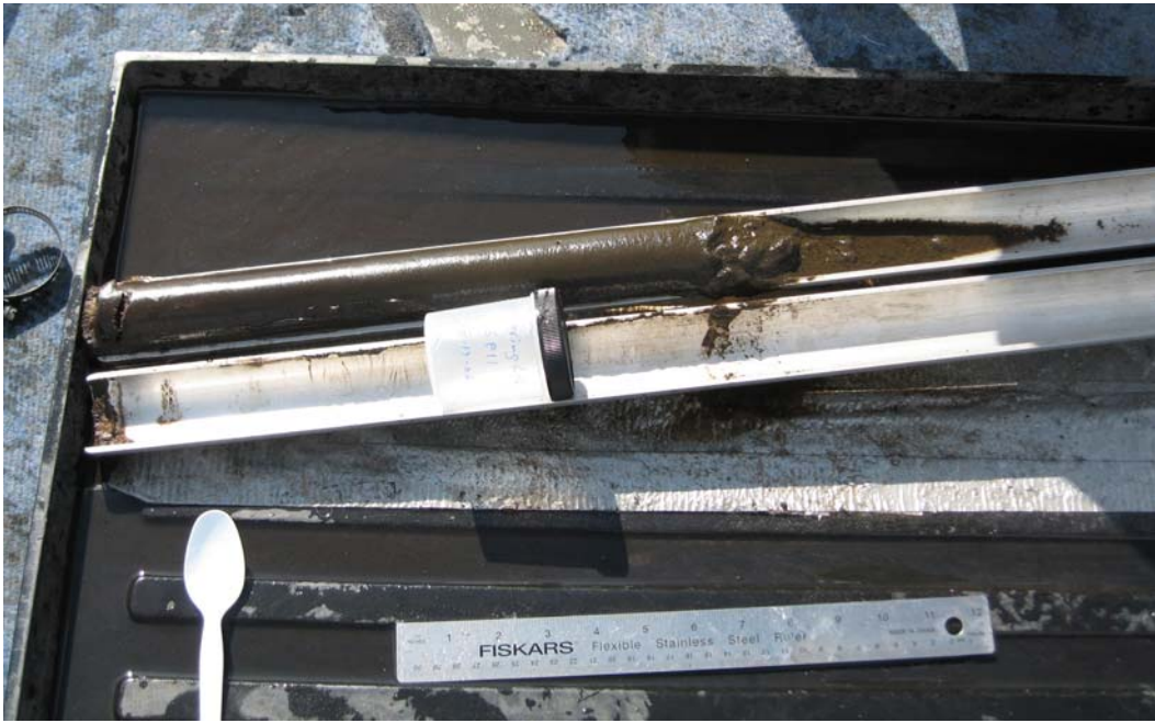
Figure 2-4a. Core Sample with Unconsolidated Organic Sediments.
