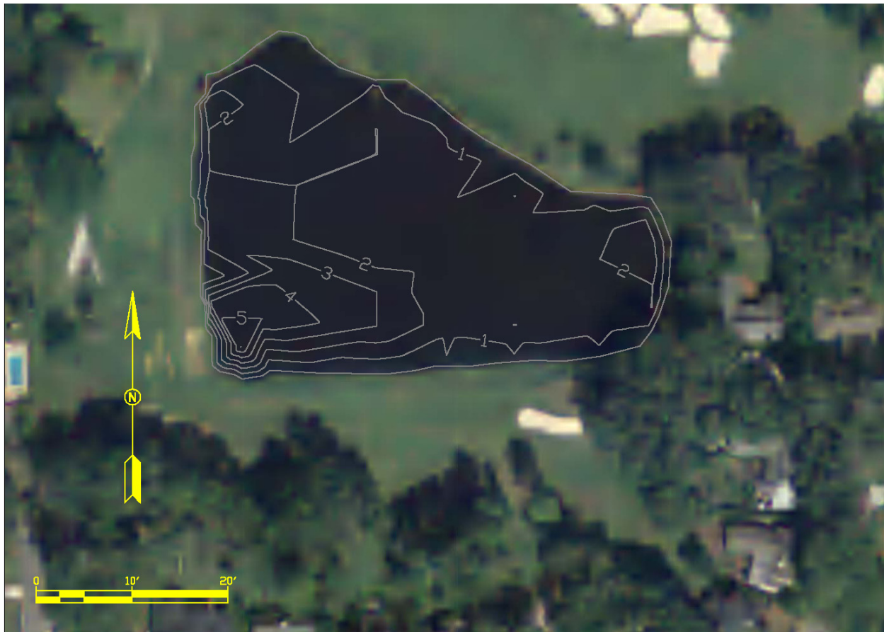
Figure 7-2. Approximate Depth Contour Map for the Sub-basin 3 Wet Detention Pond. (data collected on 11/29/07)
