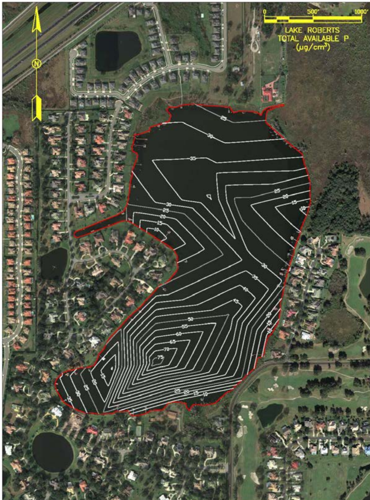
Figure 6-1. Isopleths of Total Available Phosphorus ( \mu\text{g}/\text{cm}^3 ) in the Top 10 cm of Sediments in Lake Roberts.
