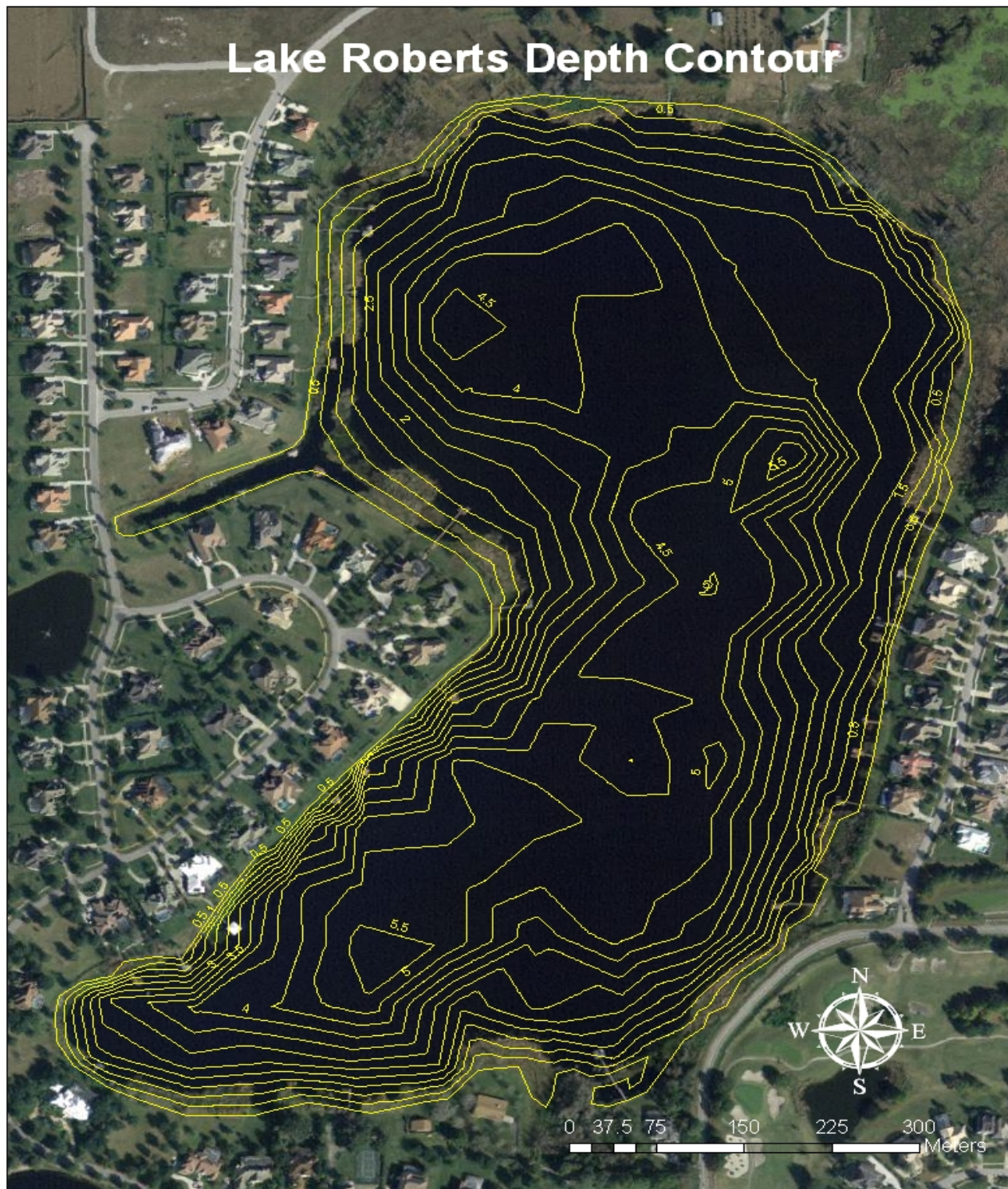
Figure 5.4. Bathymetric map generated for Lake Roberts using ArcGIS. Each contour line represents a 0.5-m depth interval.
