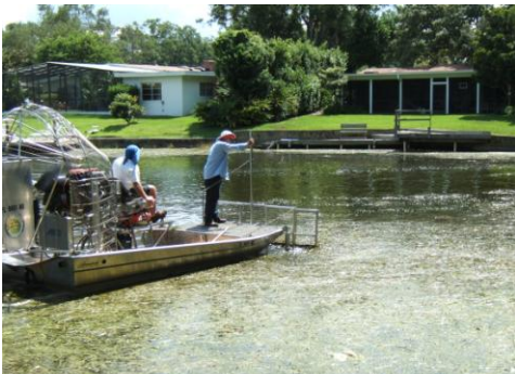
Airboat rake used to remove floating plants.
