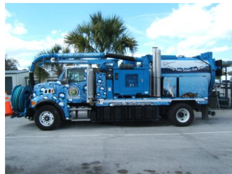
The Vacuum truck is used to maintain stormwater treatment
