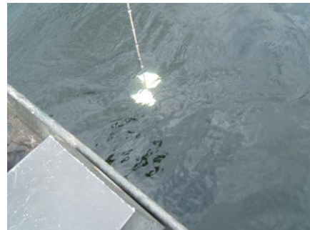
Secchi disk used to measure water clarity.
